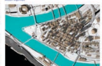
Sun and shade studies on building heights and block pattern to determine areas for housing, open spaces, and street trees
