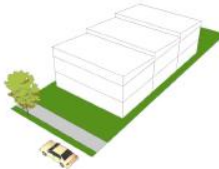
Sixplex (Stacked; Front-Middle-Back) Housing Type Spectrum: G Notes: This configuration is best suited for corner lots that allow the middle and back units to be accessed from the side street.
